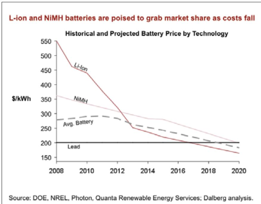
A number of factors may hold back Li-Ion adoption in SPL devices, including the need for more expensive electronics (e.g., charge controllers) to ensure safety, charge indicators to avoid over or under-charging, and most significantly, the current lack of easily available Li-Ion battery replacements in African markets. Nonetheless, the mobile market saw Li-Ion batteries take substantial share from NiMH while facing many of the same issues.
